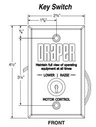
Size of wall masonry boxes required for single and key switch AII Boxes: 2" (w) x 3 ¾" (h) x 2 ½" (d)
